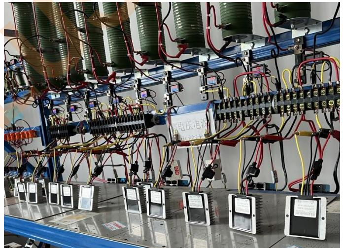
Customized products need to be tested on an aging test bench before they can be shipped.
